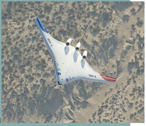
Boeing engineers say that their X-48B Blended Wing Body concept (shown here during its 50th test flight) is about 30 percent more fuel efficient than a conventional airplane of similar size that carries the same payload.
